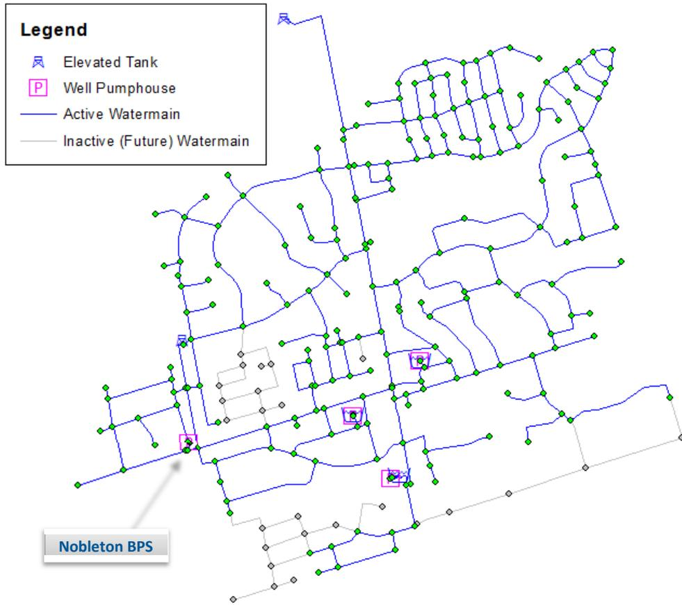
Figure 6: Updated Model – Pipeline Network
