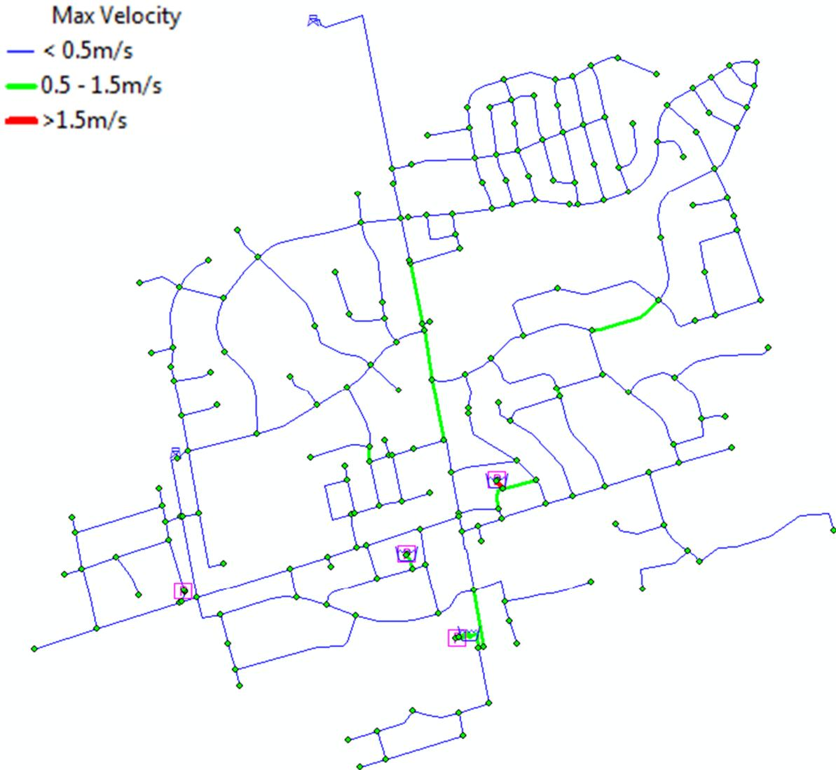
Figure 12: Increased Well Flow (6.956ML/D) Scenario – Maximum Velocity
