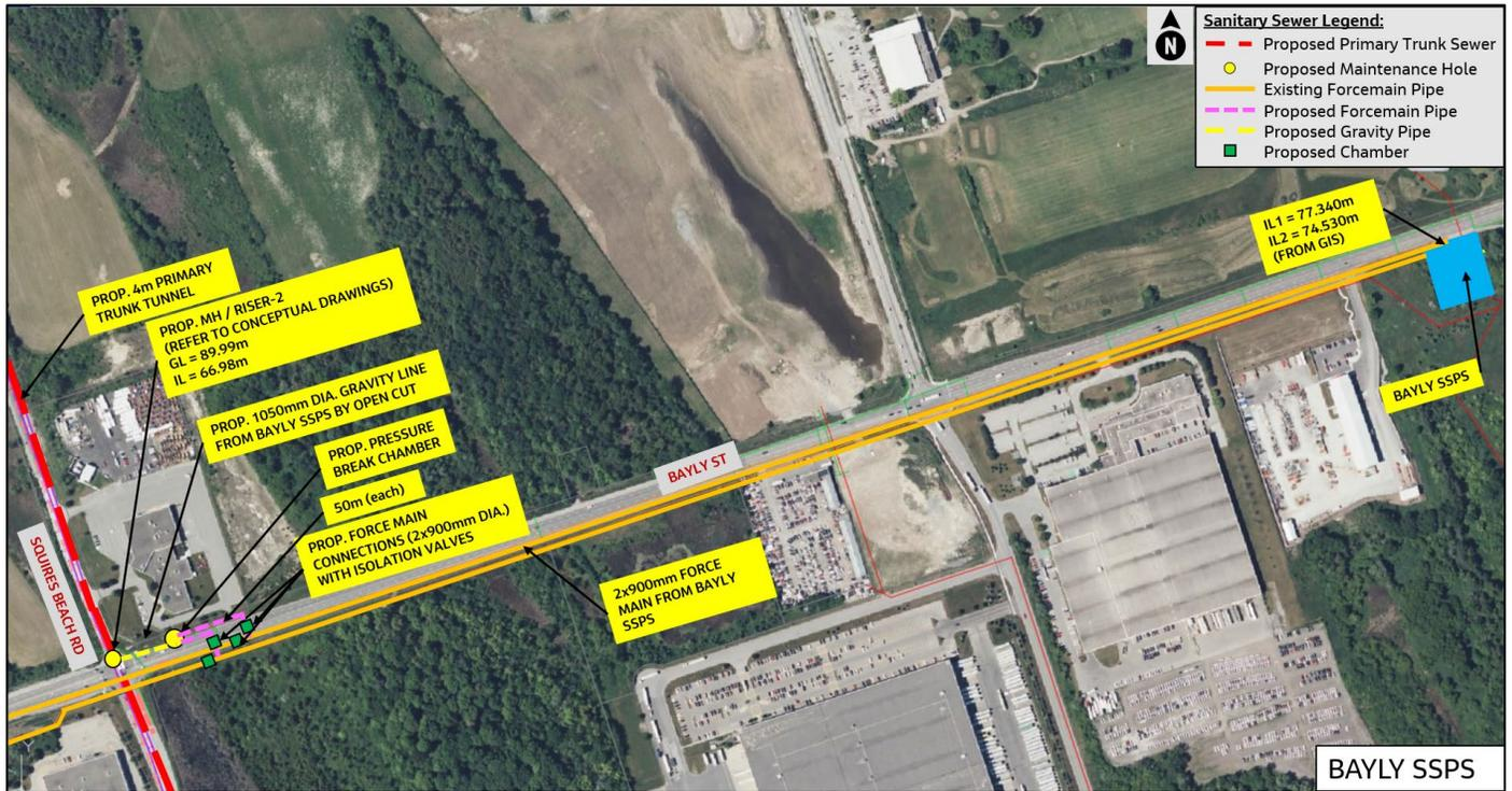
Figure 8.14 Connection of Bayly SPS to the Proposed Primary Trunk Sewer
