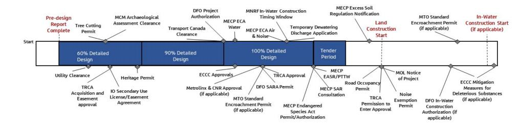
Figure 7-12 Typical Permits and Approvals Timeline for the Markham Collector Twinning Project
