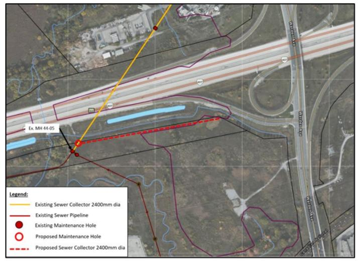
Figure 7-9 Proposed Upstream Connection Near Existing MH44-05
