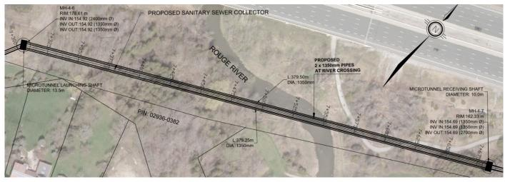
Figure 7-10 Conceptual Alignment at Rouge River Crossing
